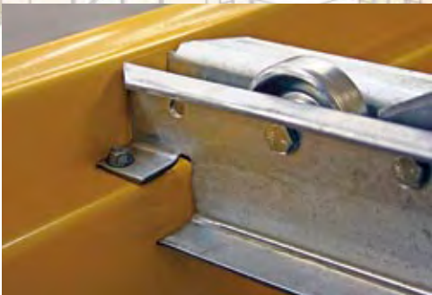
Pallet flow rails are notched to rest on the step of the beam for a lower profile that protects ends of flow rail
