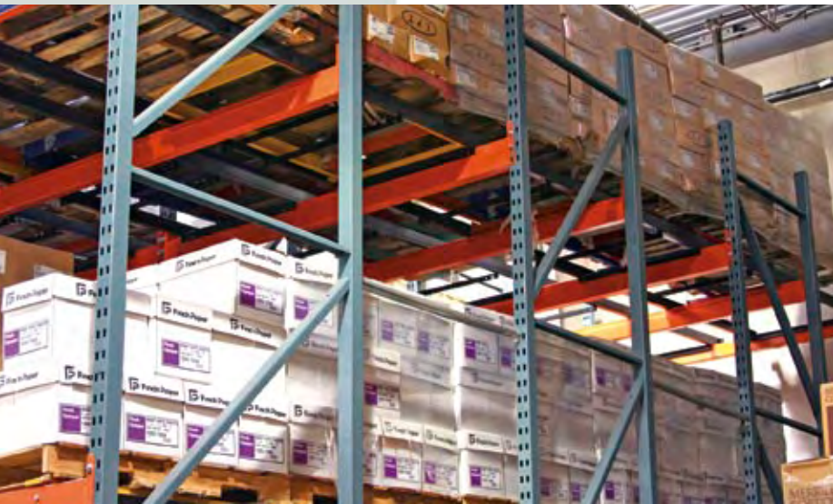
Product loads flow automatically to front picking position.
