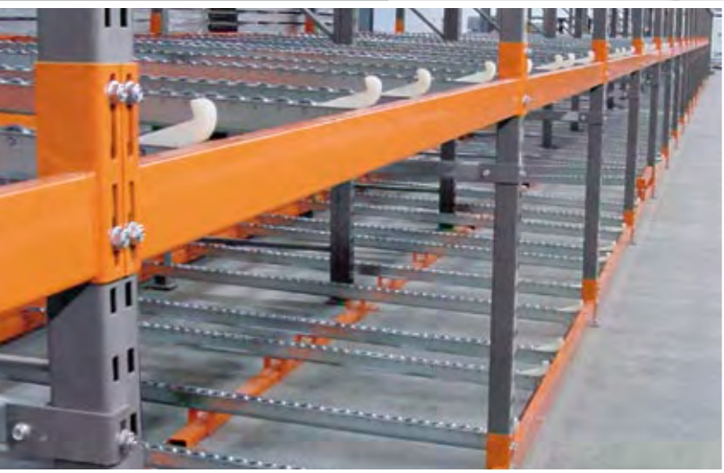
Pallet flow rails are notched to rest on the step of the beam for a lower profile that protects ends of flow rail
