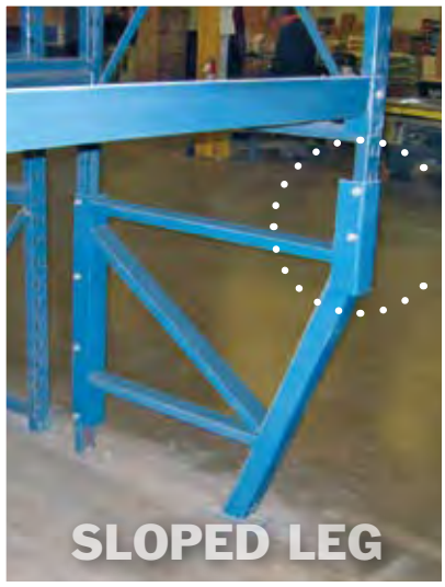
SLOPED LEG Bolt-on sloped leg option gets the upright out of the forklift traffic path to prevent repetitive damage.
