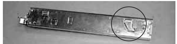
Figure 15 Slide Detail Showing Large hook
