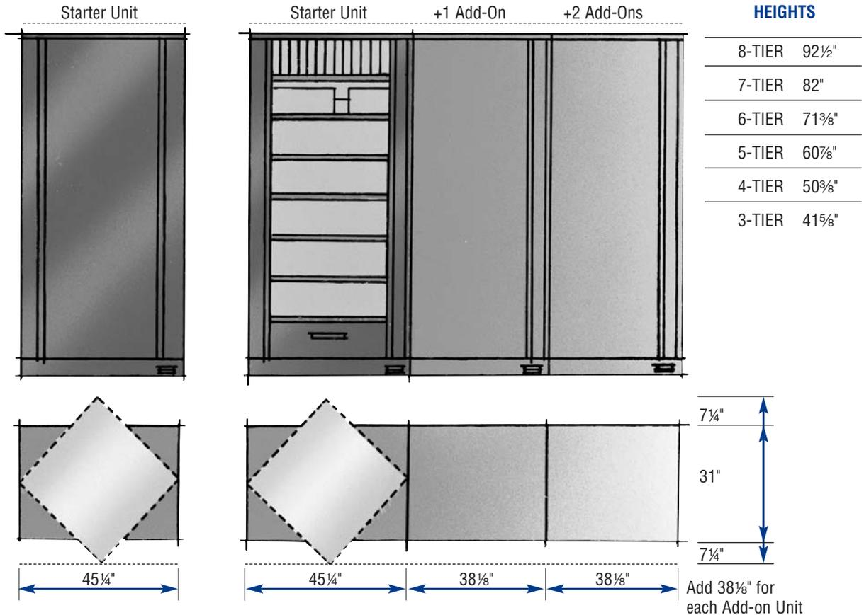
By knowing how many louvers are necessary to accommodate certain filing applications, the inside of Times-2 Speed Files becomes easy to plan. The two following charts show available size openings and the number of louvers in each height unit.
